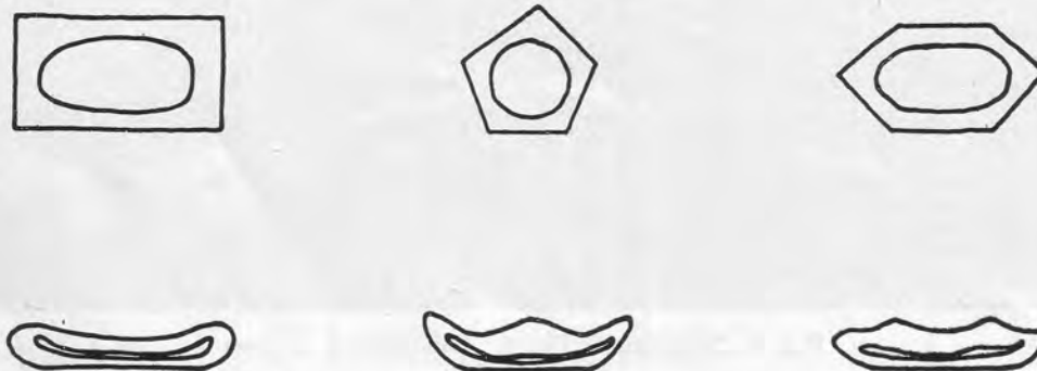
Fig. 4—Effect of collapse during drying on topography of fibres, after Emerton (3)
