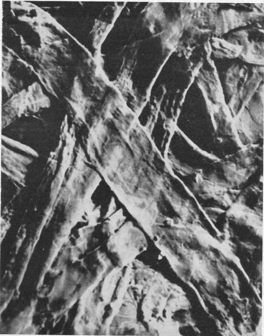
Fig. 1 —Surface of spruce sulphite handsheet (metal-shadowed replica) [ \times 650 ]
