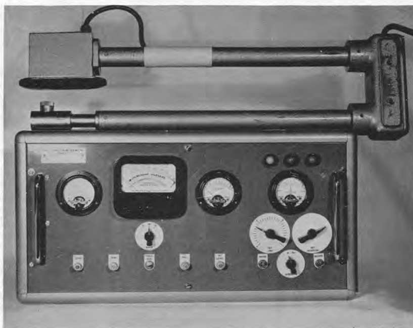
Fig. 11—The W.T. formation meter measuring head and control unit
