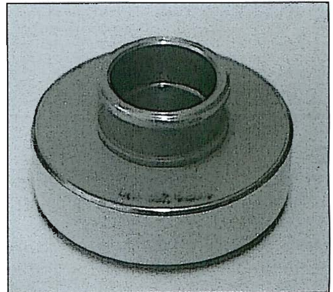
Figure 1 Metal disk matching a print disk design with a resin coating applied to the external protruding face of the hub and side surface to achieve a high friction coefficient. The unprinted contact strip is applied to the surface by double-sided adhesive tape.
